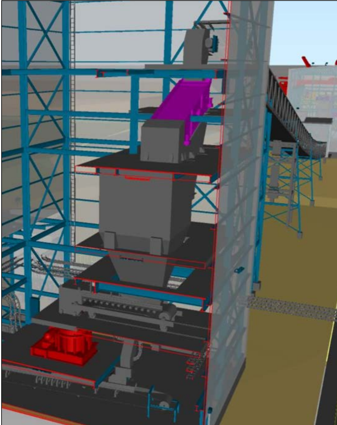
Figure 17-5 Secondary Crusher and Screen – 3D Model
